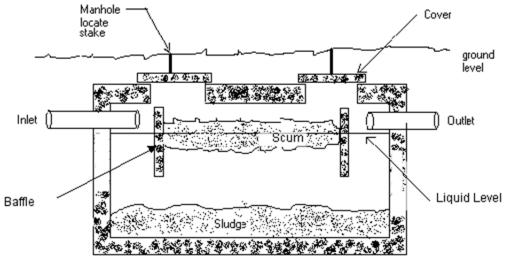
Cross Section of a Typical Concrete Spetic Tank
